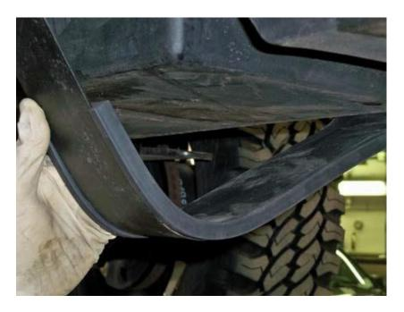
(Fig. 6) Install Rubber Strap Bushings in tank mounting strap. Center the bushings in the bottom of the straps.
